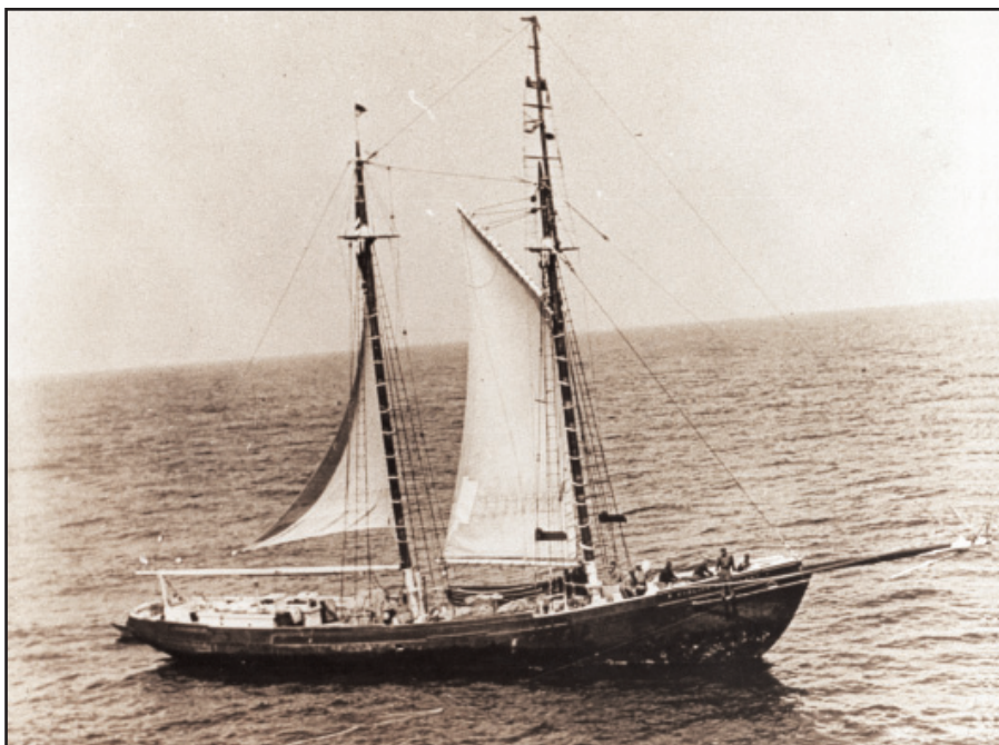
At sea in swordfishing mode: note the bowsprit with the cast iron pulpit, where the striker would stand to harpoon swordfish, and the crow's nest aloft on the foremast, where lookouts were posted to spot the fish. The bowsprit was only carried during the summer swordfishing season. Transitional schooners like the Goulart were powered by diesel engines and did not carry headsails. The foresail and the riding sail on the main mast were mostly used to steady the vessel at sea.
